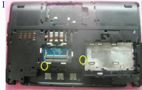
Remove 2 screws (M2.5*10mm)
