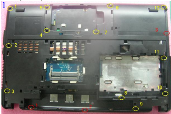
Remove screw on logic lower
