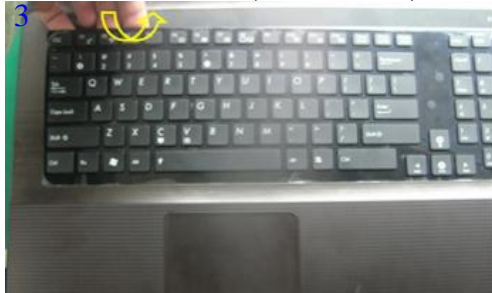
Disassemble the K/B use hand as picture shown
