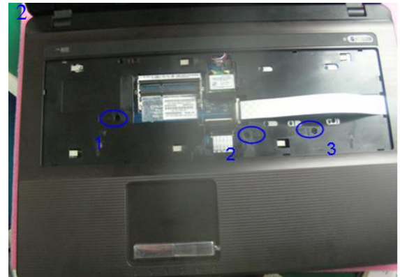
Remove screws on logic up
