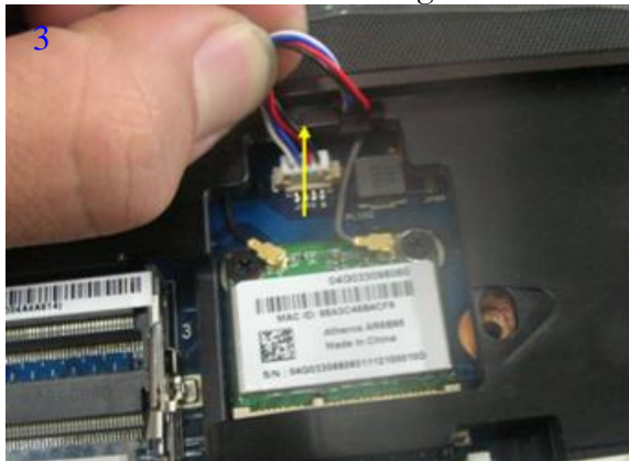
Disassemble the speaker cable follow order
